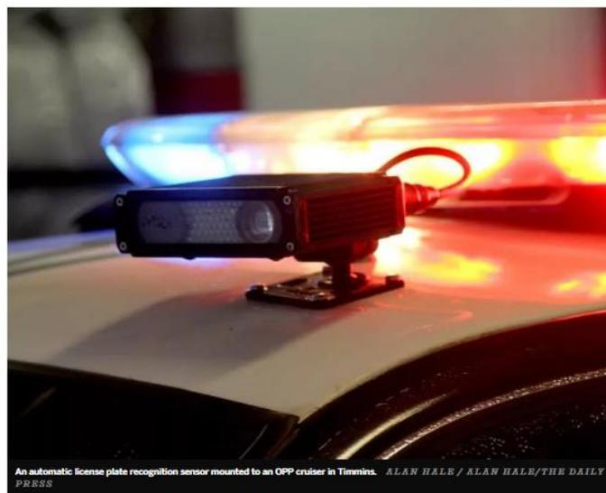
An automatic license plate recognition sensor mounted to an OPP cruiser in Timmins. ALAN HALE / ALAN HALE/THE DAILY PRESS
